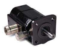
AP-HL is a HI/LO cast iron Hydraulic Gear Pump with a max pressure of 900 psi for the low pressure pump and 3000 psi for the high pressure pump. The change from LO to HI pressure is automatic with the LO side pressure pre set from 400 psi to 900 psi. The HI/LO section of the pump and the end plates are cast iron.
